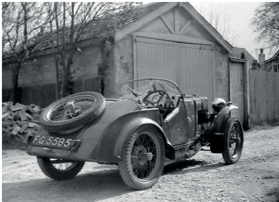
The duck’s back body on FG 5585 shown to good effect in this three-quarter rear view. Note the rear-hinged doors and external rod front brakes, identifying this as an early Oxford-built M Type.
